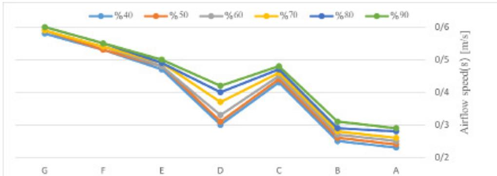
Fig. 15. Airspeed Change in Certain Points of the Studied Building at Different Angles: 90%, 80%, 70%, 60%, 50%, and 40%
