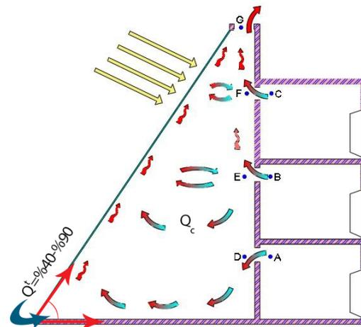
Fig. 13. Airflow Path and Heat Exchange, and Analyzed Points in a Studied Building in Kerman
