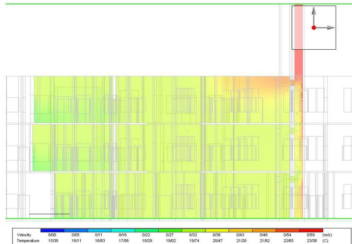
Fig. 12. Thermal Performance and Temperature Distribution and Chimney Airflow in Sample Building of Kerman
